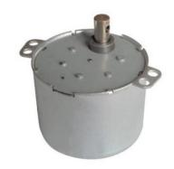
The ACPMGM AC Synchronous Gearmotors are ideal for applications that require a constant speed while connecting to the AC power line voltage. Wire up the motor with the included capacitor to the ac voltage, and the motor will maintain a constant speed as long as the load remains under the Rated Torque as listed below.
